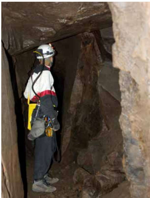
Fig. 7 - Explosives had to be used elsewhere in the inner parts of the adit when phonolitic-like rocks were encountered, as they are hard to drill conventionally (photo: D. Gómez). / Si sono dovuti utilizzare esplosivi in varie parti del giacimento quando si incontravano rocce fonolitiche, difficili da perforare in maniera convenzionale (foto: D. Gómez).
